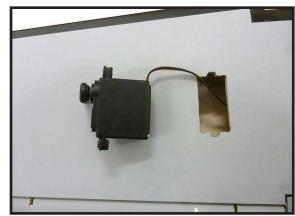
Set the aileron hatch in place and use a Phillips screw driver to install it with four
