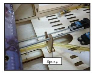
Use medium CA to glue the pushrod standoff to the inside of the fuselage and the pushrod tube.
