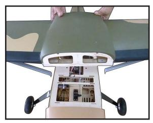
Then, install struts on the wings and fuselage.
