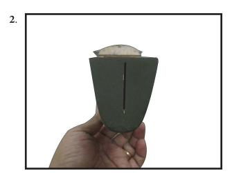
While holding the vertical stabilizer fimly in place, use a pen and draw a line on each side of the vertical stabilizer where it meets the top of the fuselage.
