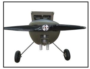
The propeller should not touch any part of the spinner cone. If it does, carefully trim spinner cone opening until propeller no longer comes in contact with it.
