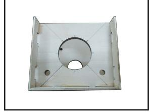
Attach the motor mount to the front of the electric motor box using four 5mm blind nut, four M5x25mm hex head bolts to secure the motor.
