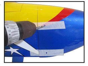
Install the muffler and muffler extension onto the engine and make the cutout in the cowl for muffler clearance. Connect the fuel and pressure lines to the carburetor, muffler and fuel filer valve. Secure the cowl to fuselage using the M3x12mm socket head screws.Putting a small length of silicon fuel tube under the head of the screw helps with vibration.
