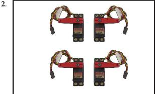
Minimum servo spec. Torque : 333.00 oz-in (23.98 kg-cm) @ 6.0V; oz-in (29.02 kg-cm) @ 7.4V
