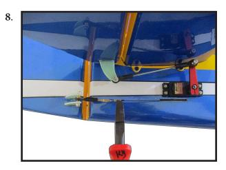
Cut off excess cable as shown.
