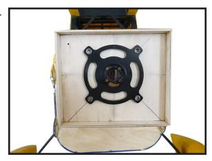
Then, use 8mm drill bit to enlarge the holes on the electric motor box.
