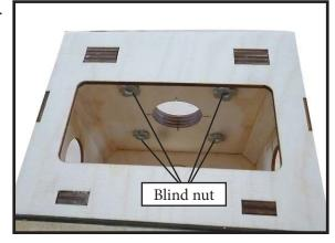
Attach the motor mount to the front of the electric motor box using four 4mm blind nut, four M6x25mm hex head bolts to secure the motor. Please see picture shown.
