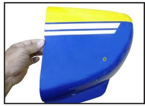
Tape the cowl to the fuselage using low-tack tape.
