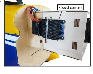
Attach the speed control to the side of the motor box using two-sided tape and tie wraps. Connect the appropriate leads from the speed control to the motor. Make sure the leads will not interfere with the operation of the motor.
