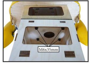
Attach the motor to the front of the electric motor box using four 4mm blind nut, four M6x35mm hex head bolts to secure the motor. Please see picture shown.
