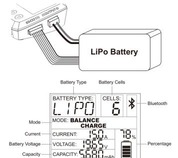
Battery Type: select the chemistry of the battery to be processed.
