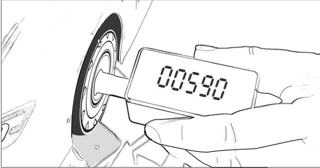
\* The viscosity of diff oil is sensitive to temperature. So temperatures variations can affect the measurement values. It is suggested to make the tests with similar temperatures environment.
