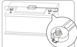
Connect the RED terminal to the positive pole, the BLACK terminal to the negative pole, or a suitable vehicle earth point. Clean the surface before pasting and fix the product body with double-sided adhesive tape.
