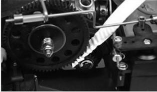
Slide a strip of thin note paper between the spur gear and the clutch bell gear. Push the clutch bell gear against the spur gear and tighten the 3x8mm adjusting plate screws. Remove the paper; the gear mesh should be correctly adjusted.
