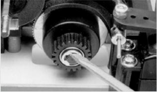
Remove the large E-clip on the clutch shaft and the clutch bell gear. Remove the ball bearings and install them in the new clutch bell gear. Reinstall the clutch bell gear and E-clip.
