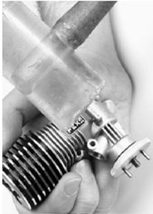
with a non-marring hammer (plastic or wood). Several easy blows may be necessary to release the flywheel and split beveled cone.
