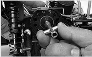
Remove the 4mm nylon locknut and the spring from the slipper clutch. Try to remove the slipper clutch as one assembly by holding the pressure plates together with your thumb and index finger.
