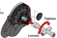
slipper clutch plug on the transmission cover in order to adjust the slipper. Use the 4-way wrench to turn the adjusting nut clockwise to tighten and counterclockwise to loosen. Place the model on a hightraction surface, such as carpet. Adjust the slipper so that you can hear it slip for approximately two feet from a standing, full throttle start. (Learn more about adjusting the slipper clutch in the sidebar.)
