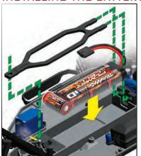
Install the battery pack with the battery wires facing the rear of the model. Insert the tabs of the battery hold-down into the slots in the rear hold-down retainer and then place the battery hold-down over the post. Secure the battery hold-down with a body clip in the hole in the post. Do not connect the battery pack yet.
