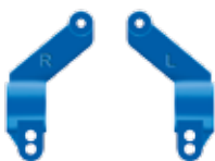
Aluminum axle carriers reversed: 1° toe-in
