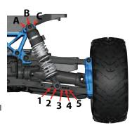
The suspension of your model has been set up for off-road performance (position 2 on the front suspension arms and position 3 on the rear suspension arms). If you plan on driving on hard surfaces, the following changes should be made:
