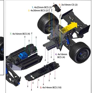
• When reinstalling the motor, ensure that the gear mesh pins are in the correct locations (refer to the pin location chart on page 24). Place the motor onto the rear bulkhead and install the gear cover with the 3x10mm cap screws (2). This will allow the truck to be flipped upside down and still maintain proper gear mesh. Flip the truck upside down and install the 4x16mm button-head cap screws (4) into the motor mount.
