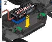
**Note:** The battery compartment will accommodate the Traxxas 6700mAh 4s battery pack (part #2890X). When using other LiPo batteries, additional foam blocks and battery pack spacers are required for proper fitment (*see battery chart*).
