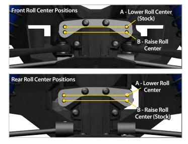
Note: If you place the front links in the bottom position (not stock), then the pivot balls in the steering will need to be flipped. The outer pivot balls come out of the box in the lower position (A). When the roll center is moved, the offset will need to be flipped (B).
