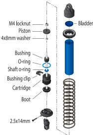
**Note:** The new cartridge must be assembled on the shock shaft. DO NOT attempt to assemble the cartridge separately and slide it onto the shaft. This may damage the shaft O-ring and cause a leak.
