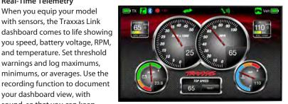
The customizable Traxxas Link dashboard delivers real-time rpm, speed, temperature, and voltage data.
