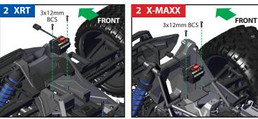
Install the high-voltage power amplifier on the truck chassis. Ensure that the connectors on the amplifier face the front of the vehicle. Secure with the 3x12mm button-head screws.
