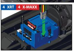
Plug the 8-pin connector from the high-voltage power amplifier into the accessory port on the ESC. The amplifier and lights will turn on when the ESC is powered on.
