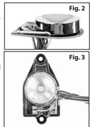
3 Install the circuit boards into the existing plastic headlight mounts (H);
