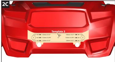
Peel the adhesive backing from **Template 3**. Place the template on the body (**2C**), aligning the bottom of the template with the holes in the body cut using Template 2 from the previous step. Using a tapered body reamer, carefully cut holes in the body to the dotted lines on the template. Use body scissors to cut out the section between the six holes, along the dotted lines as indicated
