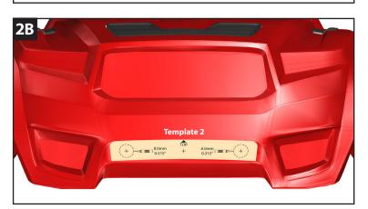
Peel the adhesive backing from **Template 2**. Place the template on the front of the body as shown, using the body lines for alignment **(2B)**. Using a tapered body reamer, carefully cut holes in the body to the dotted lines on the template.
