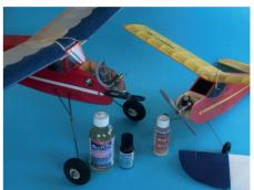
will ensure that the trim is fuel proofed. Loose Monokote trim used on this KK Bandit fuselage was sealed successfully with Aerokote.
