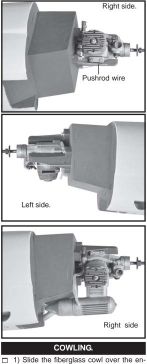
□ 1) Slide the fiberglass cowl over the engine and line up the back edge of the cowl with the marks you made on the fuselage.
