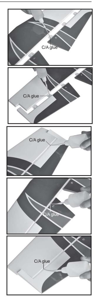
$\Box$  1. Draw a center line onto the horizontal stabilizer. Then slide the horizontal into the fuselage.
