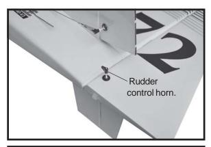
RUDDER PUSHROD INSTALLATION.
