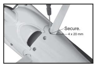
□ 2) Using the hardware provided, mount the main landing gear to the fuselage.
