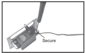
$\Box$  5. Instal servo tray with aileron servo into the wing as same as picture below.
