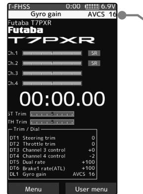
The value of the gyro gain is indicated to the top of the screen for several seconds.
