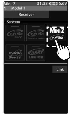
**2** Touch [Link] on the transmitter T7PXR screen, you will hear a chime sound, and T7PXR will enter the link mode for 20-seconds.
