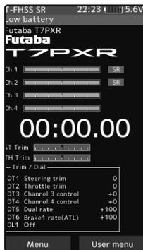
If the transmitter battery voltage drops below the usable range, an audible alarm will sound and "Low battery" will be displayed. Since the usable range of LiFe and Ni-MH batteries are different, the power supply used must be set by the system setting.
