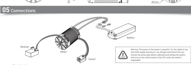
Insert the throttle cable of the ESC into the throttle channel of receiver (that's THROTTLE channel). Because the red line of throttle cable output 6V/7.4V voltage to receiver and steering servo, do not supply power to receiver, otherwise the ESC may be damaged. If need to supply power, pick out the red line among throttle cable, wrap it and suspend
