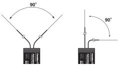
The two antennas should be placed at 90 degrees to each other.
