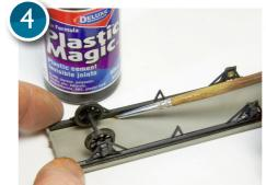
The new formula of Plastic Magic works quicker and more effectively than its predecessor and is best applied by fine brush or Pin Flow applicator, added sparingly into the joint while the parts are pressed together.
