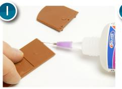
After fettling the parts and undergoing a dry run to ensure that everything fits together cleanly. Roket Plastic Glue is best applied with the supplied needle tip to both parts. Run a thin bead of glue along the joint faces.
