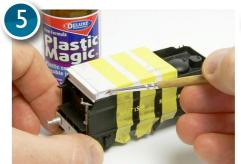
A good test of Plastic Magic's ability is to try and bond styrene to the tough plastic used on RTR models, such as this Bachmann tender. The powerful solvent formed an extremely strong bond.
