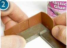
Gently press the two parts together, ensuring that they're correctly aligned, using a setsquare if necessary. The glue takes a few seconds to 'grab', so make any necessary adjustments and set aside to cure.
