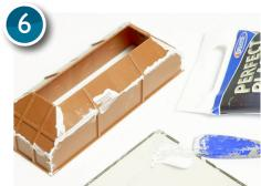
Perfect Plastic Putty is best decanted onto a sheet of plastic or glass before applying to the model with a plastic spatula. It spreads easily and dries quickly. Build up the putty so that it's slightly above the seam.
