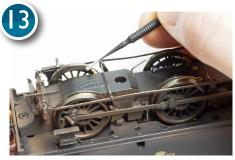
The microbrush, soaked in Track Magic, will remove debris, dirt and oil deposits from the power contacts and the bearing faces of wheels and axles - an often-overlooked facet of locomotive maintenance.
