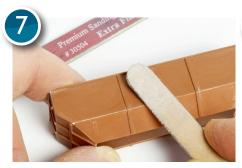
Leave aside for an hour or two before sanding flush and smooth with sticks, files or wet 'n' dry paper. Using progressively finer abrasives will polish the surface to a high sheen. Check for remaining gaps and repeat if necessary.
